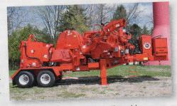
horsepower, the compact NCL model still utilizes the established 83-inch disc with three or four knives.
